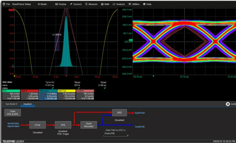
Optimize the equalizer at the receiver and see the impact on the eye diagram.
